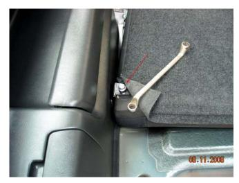
Suzuki Jimny 1.3 JLX Rear Seats Removal
