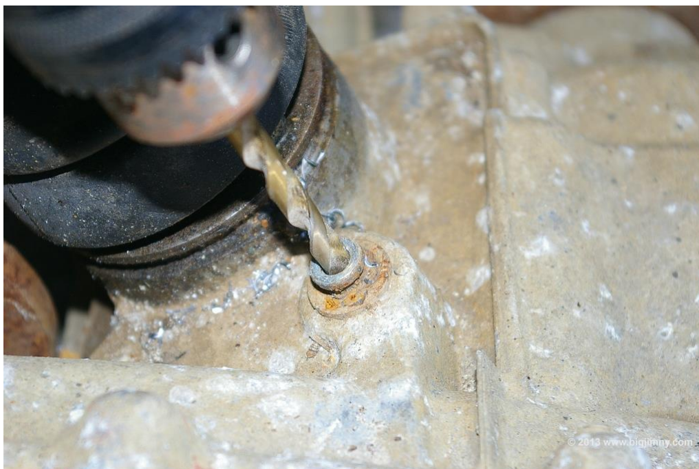
Figure 7. Drilling the Transmission box
