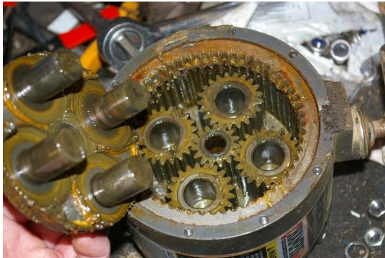
Figure 11. Layer 1 with the 4 heavy duty gears
