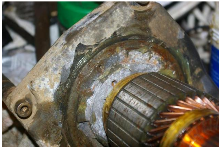
Figure 22. Greasing the frame/casing joint
