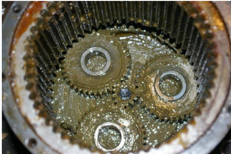
Figure 14. Layer 3 gears (the thinnest)
