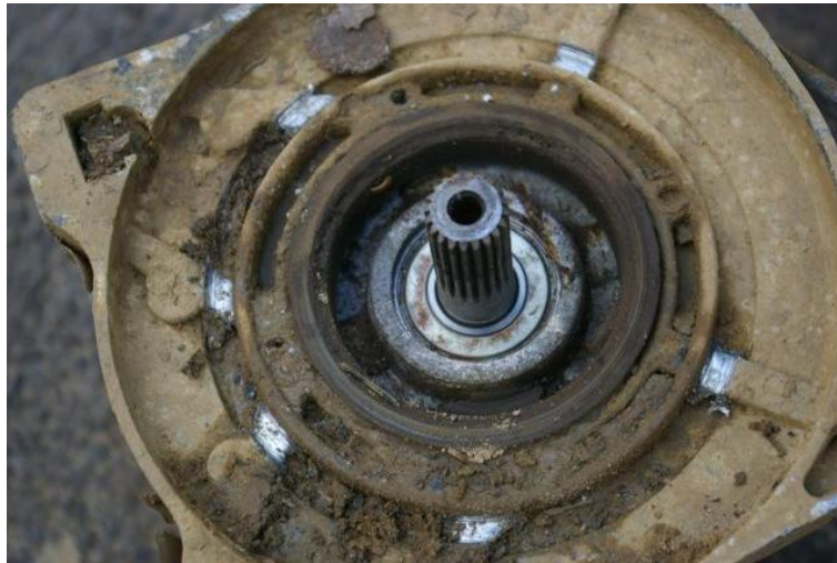
Figure 21. Motor showing bolt fouling marks
