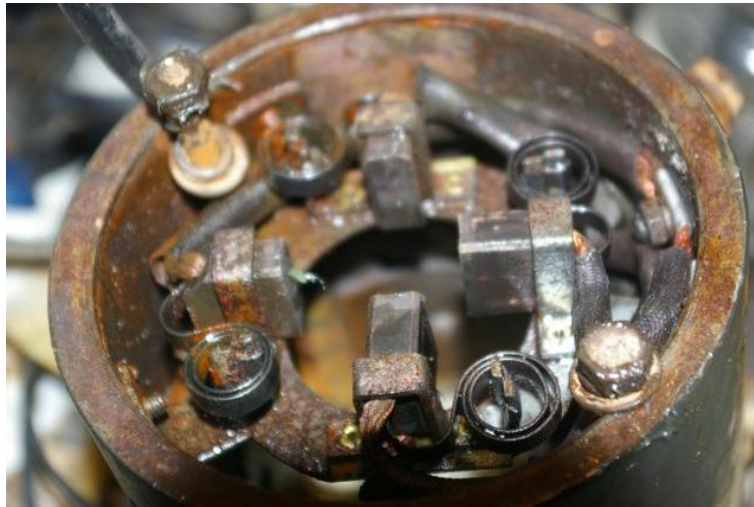
Figure 23. Motor brushes (see how the stuck ones have not sprung forward in their mounts)
