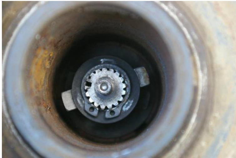
Figure 4. Drum Brake stuck in drum
