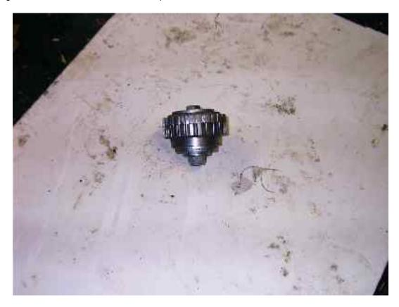
I unbolted the two gears. Then tack welded the gear to the rear TX box flange. There is a nice step in the flange which I butted the gear up to. This helped it to stay straight. I checked it was running true by fitting it to the TX box and spinning it round. When happy with it I welded it more securely.
