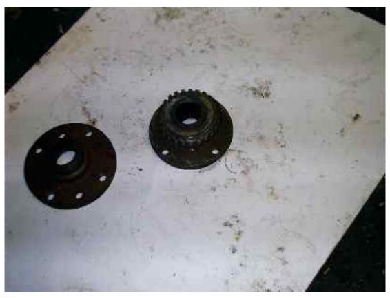
Next I used some car body filler to fill the gaps between the teeth. I also made it thicker to get it as close as possible to the TX box rear oil seal. I smoothed it off round and painted it! This was to keep the muck at bay.
