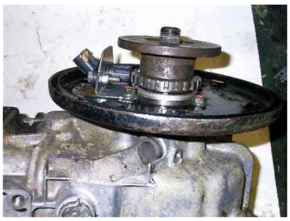
I cut away most of the backplate, leaving just enough to carry and protect the sensor.
