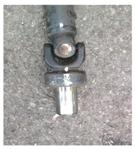
Then remove the circlips in each of the joint caps. Tapping the cap inwards can help with this.
