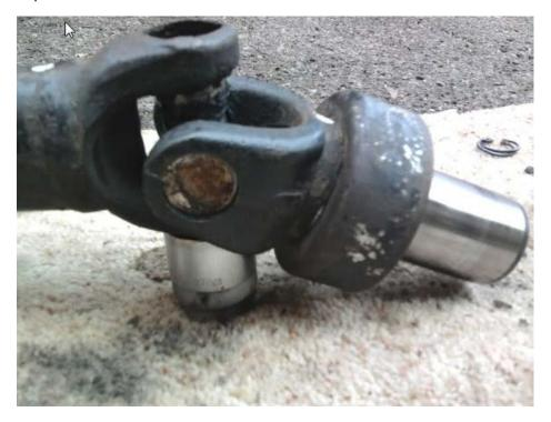
Once the end cap is completely proud of the yoke you can pull it the final few mm with mole grips if necessary
