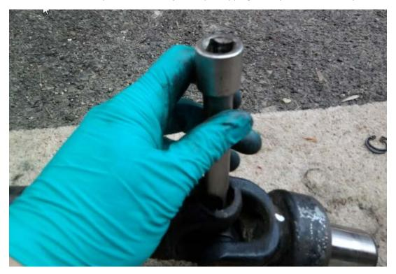
I use a ½" extension socket – fits well on top to drive the races out. A 24mm socket below the joint allows you to drive the end caps out.
