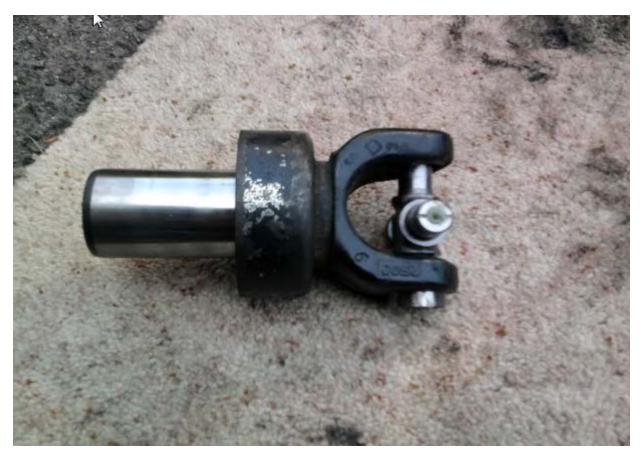
Once your first circlip in in, turn the yoke over and tap the opposing race until you can get the second circlip in.
