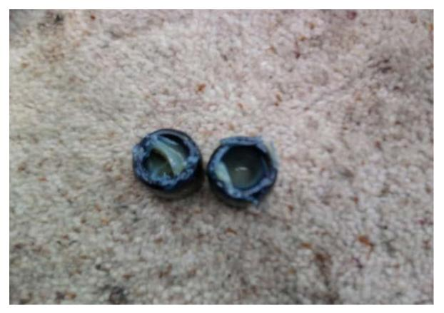
Place one into your yoke, tap it a little way in, slip the cross piece in and pop in the other race. Tap all the way in until you can fit your first circlip.
